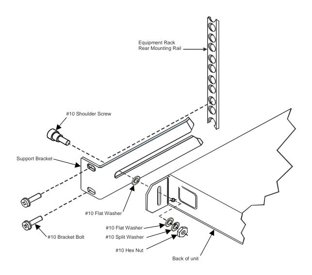
Figure 2-1. Optional Rear-Mounting Support Brackets Installation
