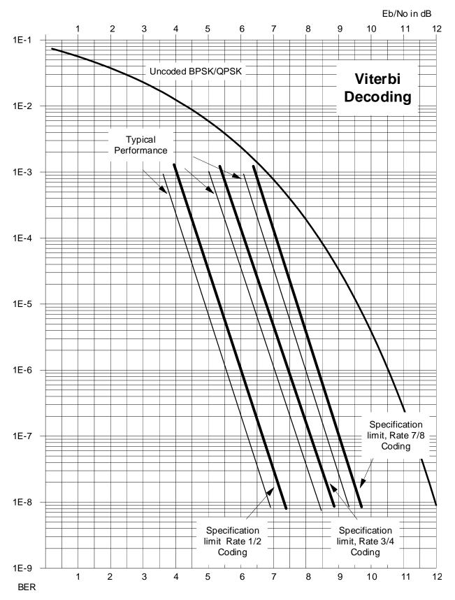
Figure 6-1. Viterbi Decoding
