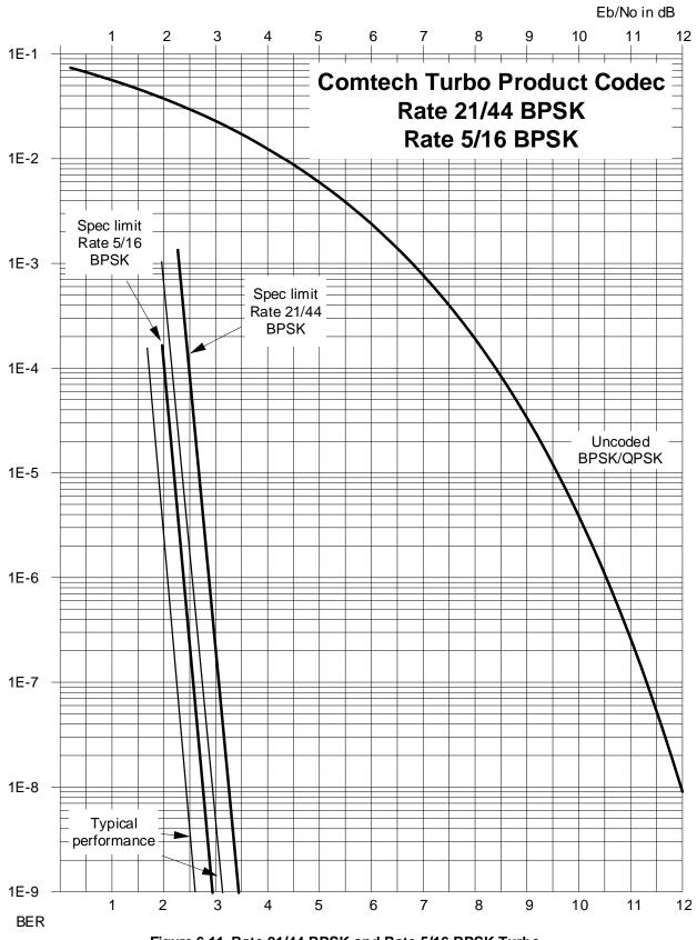
Figure 6-11. Rate 21/44 BPSK and Rate 5/16 BPSK Turbo
