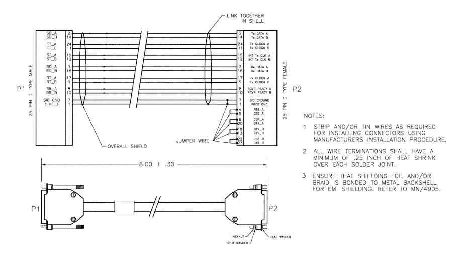
Figure A-3. DCE Conversion Cable: RS-530 (CA/WR9718-1)
