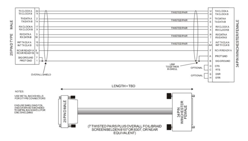
Figure A-4. DCE Conversion Cable: RS-530 to V.35
