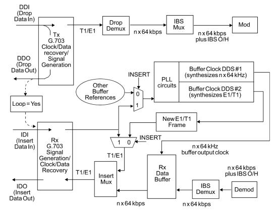
Figure 8-4 illustrates the general arrangement for Drop and Insert clocking in the CDM-600/600L.
