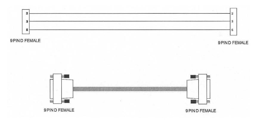
Figure A-5. Switch Programming Cable
